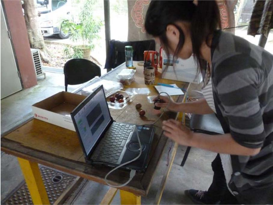
Fig. Scanning prune fruits by NIR spectrometer
