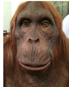
Robotic orangutan from BBC TV Series ‘Spy in the Wild’ - the right eye is a 4K spy camera
