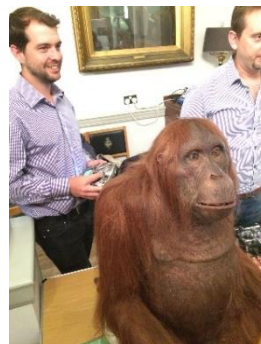
Robotic orangutan from BBC TV Series ‘Spy in the Wild’ - the right eye is a 4K spy camera
